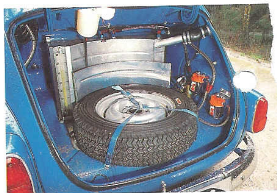
Right, beautiful 70-litre aluminium tank is situated over axle line to improve handling. Original wheels are now rare, left. Note fuel filler cap and reversing light
