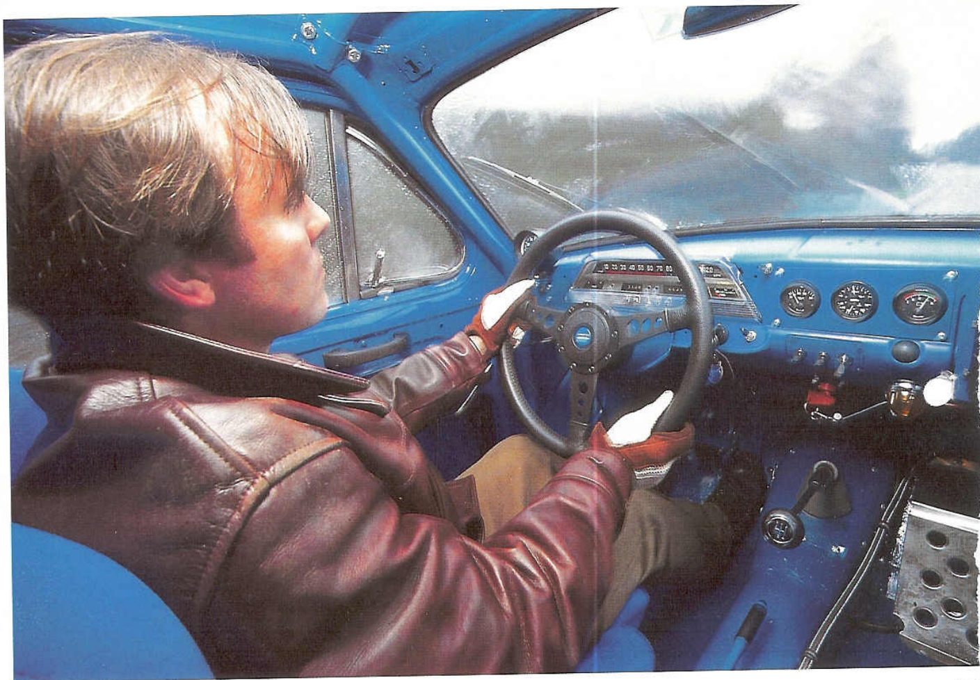
Top, stripped-out interior is beautifully finished, with custom-built cage, drilled footrest for navigator and modern instruments
